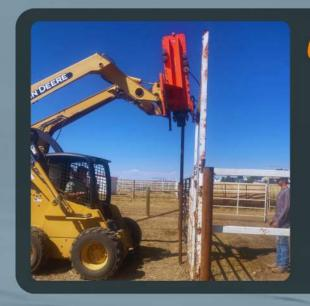
The Vibe Drive Pole-Cat has increased safety and overall efficiency of our fencing projects, especially when driving steel from T-posts up to 6 inch pipe. Driving wood we have yet to break a \$15 post.
