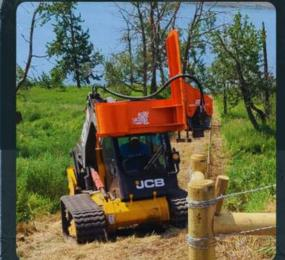
Our Timber-Wolf was being serviced, so we used our hammer pounder. Within 2 hours it splintered a new post. The operator jumped to avoid injury and stopped the job to wait for the Vibe Drive.
